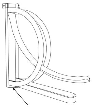
3. Drill the third hole for installation at the bottom of the single wall unit and fasten the last bolt in place using the same procedure as step 2 according to your wall type (concrete or wood).
