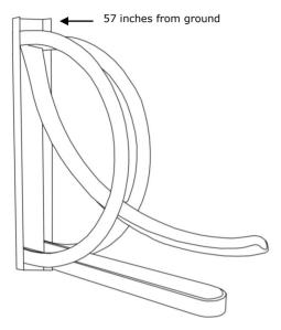
1. Hold the single wall unit against the wall for installation at a height of 57 inches (top of rack) from the floor.
