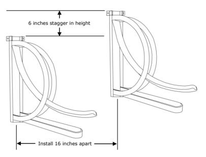
4. (Optional) To install additional racks along the same wall, repeat these steps while staggering the racks in height by 6 inches (63 inches from the floor) for every second rack, and install each rack at least 16 inches apart on center.
